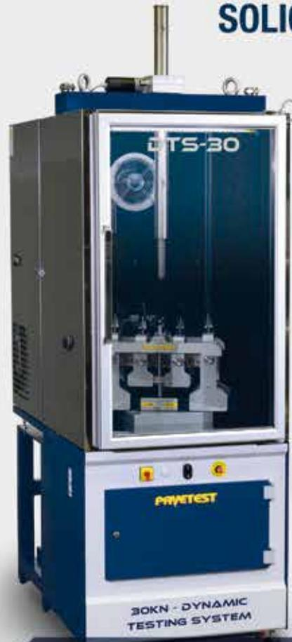
PRENSA SERVO-HIDRÁULICA 30 KN,
