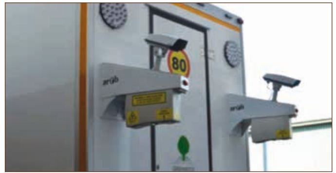
Figure 7. The ACD system installed at the rear of the trailer measures 4000 points (combined) across the lane. It also houses the rear facing asset cameras.
