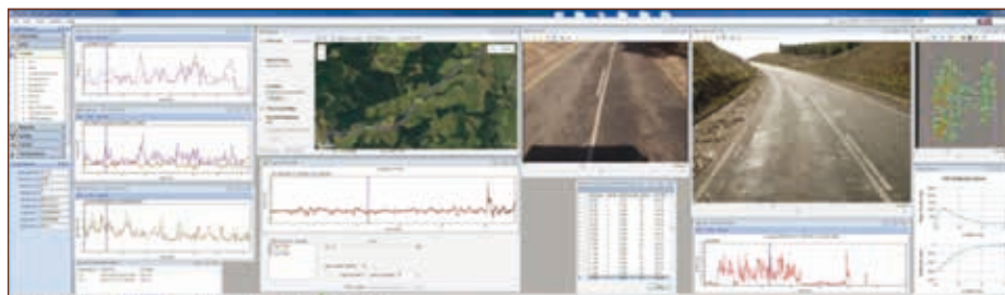
Figure 9. Screenshot of the Hawkeye processing toolkit with multiple windows displaying the integration of the several systems.
