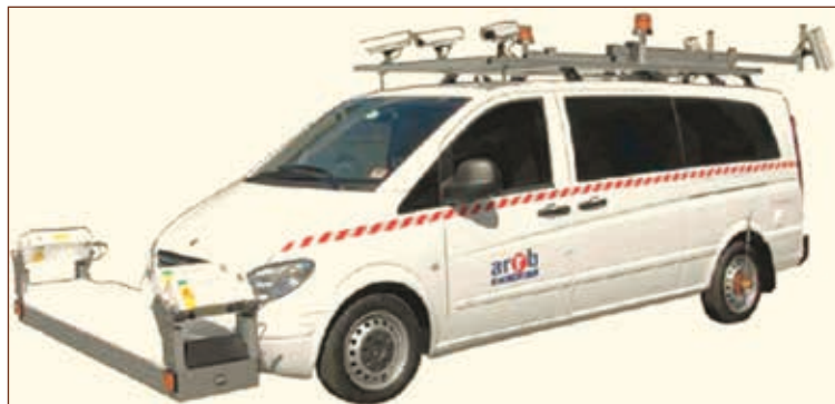
Figure 1. Example of a Digital Road Surface Profiler with an integrated imaging system.
