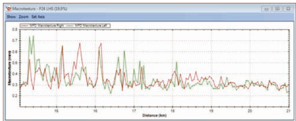
Figure 11. Screenshot of MPD texture measurements on P24 trial section.
