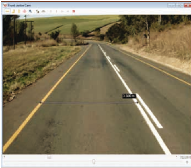
Figure 13. Example of forward facing asset cameras depicting measurement capabilities.
