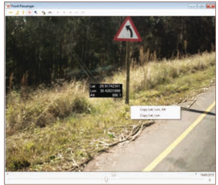
Figure 13. Example of forward facing asset cameras depicting measurement capabilities.
